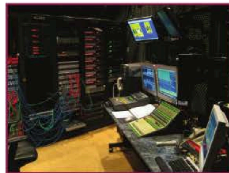
The backstage technical area housed a Meyer LCS CueConsole control surface and Matrix3 mixing system for monitoring.
